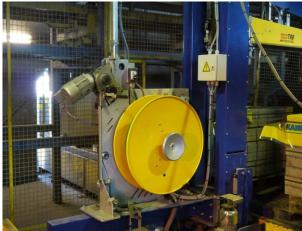
Easy to load integrated strapping dispenser with automatic strap feed and re-feed to the sealing module ensures quick, easy and reliable strap loading. Increases machine efficiency and uptime.
