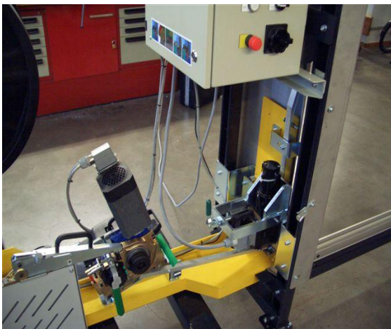
Easy access MH feed and take up and MH Strap sealer module on MH-V model
