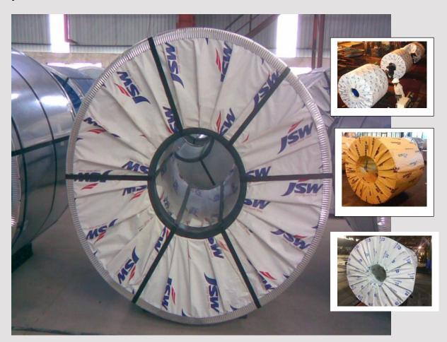
**Signode India**, a leading industrial packaging solutions provider has introduced <u>Strength Fabric</u>, <u>the superior and cost effective protective packaging solution</u> as compared to the conventional fabric in the market. Strength fabric is poly based fabric coated with polyolefin blend for high strength and product protection.
