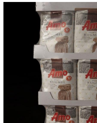
Controlled application of stretch hood film on bags with flour stacked in cardboard trays.
